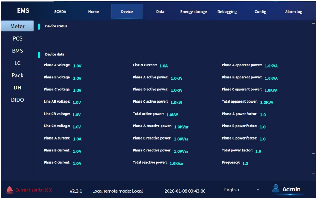
Figure 7.4-1 Power Meter Interface
